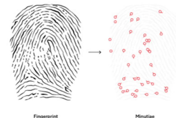
FIGURE 2. EXAMPLE OF A BIOMETRIC TEMPLATE (BASED ON FINGERPRINT MINUTIAE)
